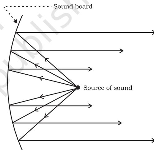
**Fig. 12.15:** Sound board used in a big hall.
