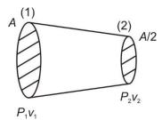
Using continuity equation between section 1 & 2
