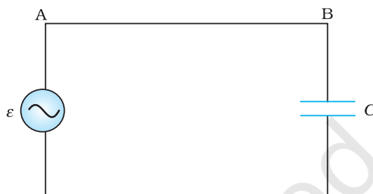
FIGURE 7.8 An ac source connected to a capacitor.
