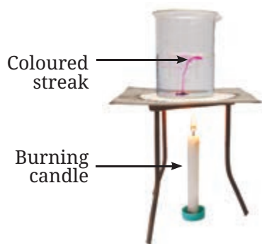
Fig. 7.5(b): Demonstration of convection in heated water
