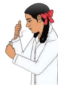
Fig. 8.19: Correct way to waft the fumes of an evolved gas
