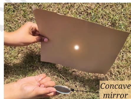
Fig. 10.12: Converging sunlight on paper using a concave mirror
