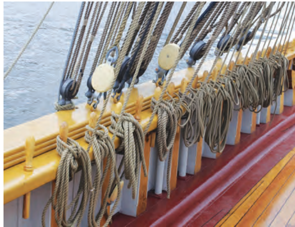
Fig. 7.21. Pulley used in boats
