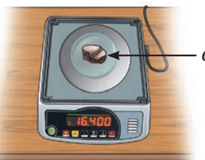
Fig. 9.12(c): Weighing a solid object on digital balance
