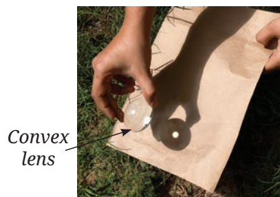
Fig. 10.19: Converging sunlight on paper using a convex lens
